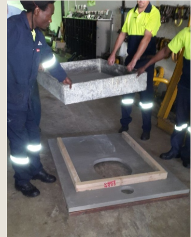
FRAMEWORK TO SIMULATE TOP STRUCTURE PLACED ON SLAB
