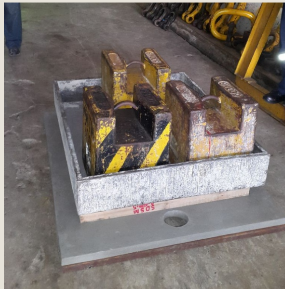
"TOP STRUCTURE" LOADED TO 1.5 TONS
