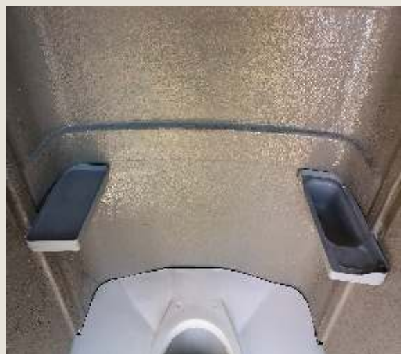
If required, bolt the shelf and hand basin into place using 4 x M6 x 20mm machine screws provided.
