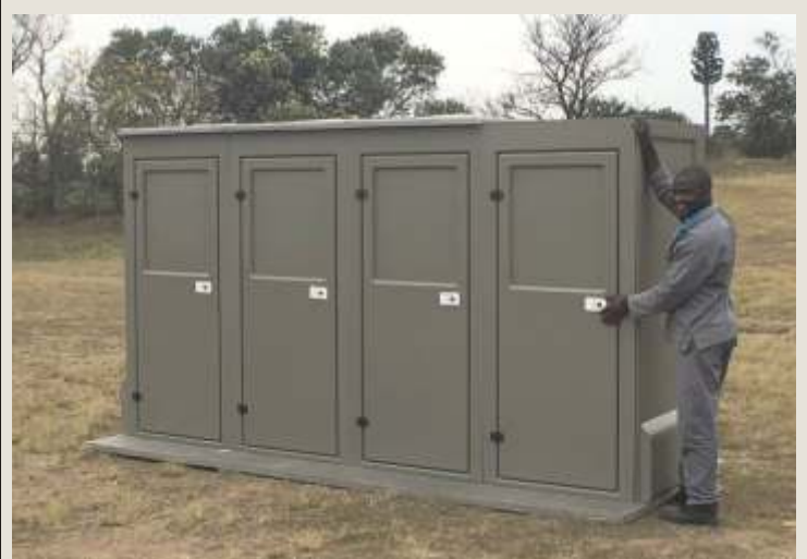
Fix the last Front Door-Wall to the previous one, aligning the left side flange of the Front Door-Wall into the groove of the Mid Wall, also fixing the right side flange to the Right Side Wall using 5 x M6 x 20mm machine screws provided and then fix down to the slab structure with suitable fixings.
